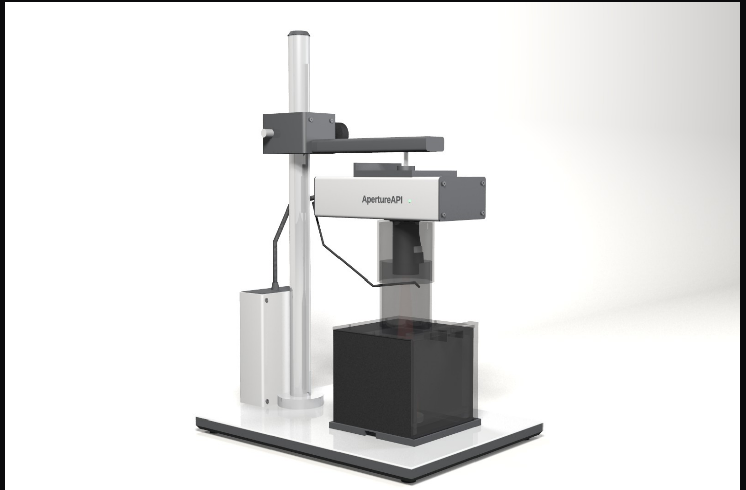
CAD render, design values; front door, lid and light sleeve shown translucent for illustration; the laser is off whenever the door is open. Hardware qualification planned. Nothing built, nothing measured; every figure in the design files is a design value.
